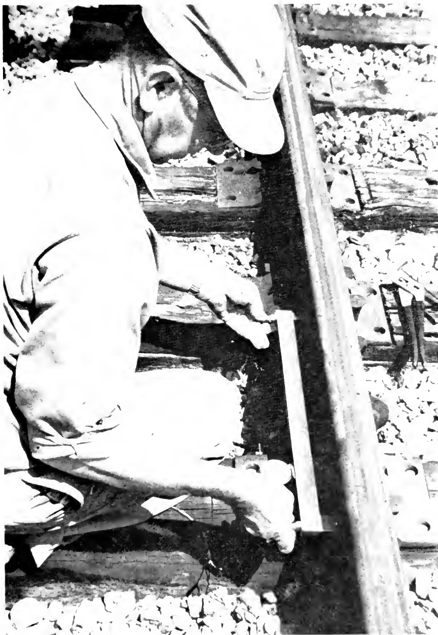
Fig. 4—Measuring longitudinal stress in rail with 20-in Berry strain gage.
